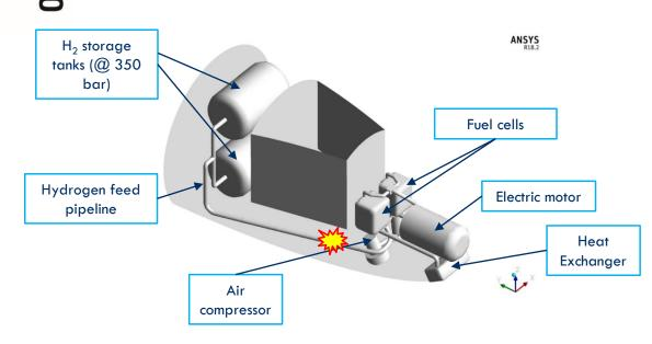
Design from: G. Romeo et al., «ENFICA-FC: Design of transport aircraft powered by fuel cell & flight test of zero emission 2-seater aircraft powered by fuel cells fueled by hydrogen», International Journal of Hydrogen Energy 38, pp 469-479, 2013.
